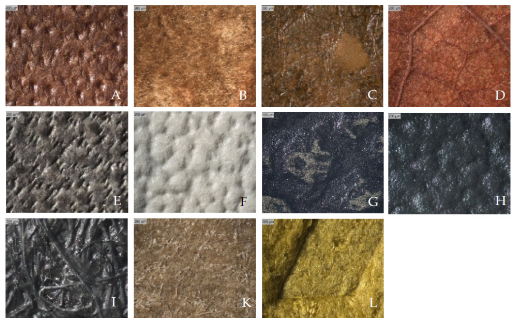
Figure 3. Surfaces of the investigated materials: Naturally grown material (Leather (A), Muskin ® (B), Kombucha (C), Teak Leaf ® (D)); embossed surfaces of coated textiles (PUR-coated textile (E), Desserto ® (F), Appleskin ® (G), Vegea ® (H)); fiber structures of non-woven natural fibers (Pinatex ® (I), SnapPap ® (K)), and micro-fiber material (Noani ® (L), embossed).
